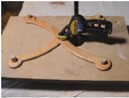
Clamping rails using the jig for positioning
