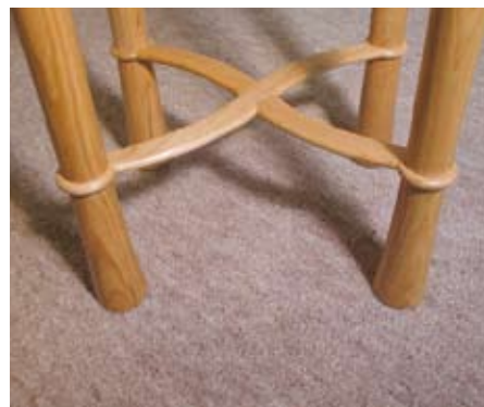
Leg bottoms and rails fitted to mid-sections
