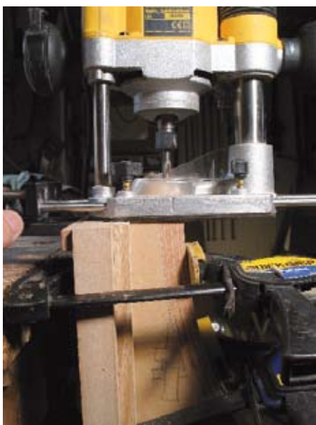
Set-up for routing the curved apron for loose tenons
