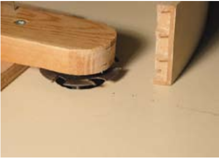
Make-shift ring fence on router table for cutting grooves in the drawer front (guard removed for photo only)
