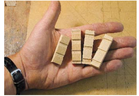
Cut packing pieces to the exact profile of the drawer and moulding in order to prevent bruising when clamping
