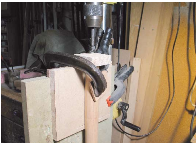
Set-up for drilling end of the leg on a pillar drill
