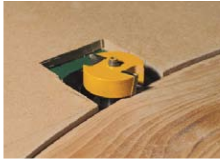
Rebate cutter and curved fence used to rebate the front of the drawer bottom (guard removed for photo only)
