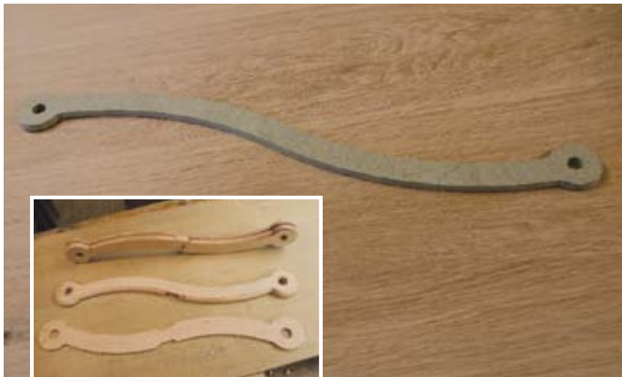
Stretcher template (main pic) and (inset) at top – rail as shaped; middle – rail with waste cut away; bottom – waste piece
