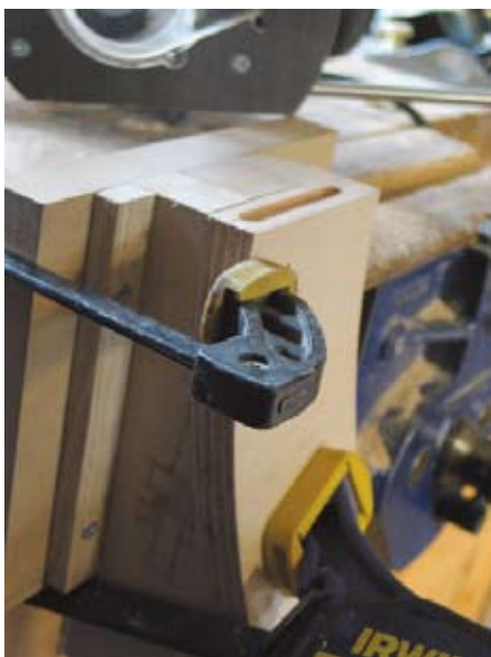
The curved apron piece in the jig showing a routed mortise
