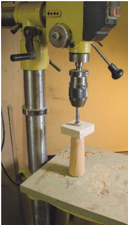
Drilling the foot to receive a dowel
