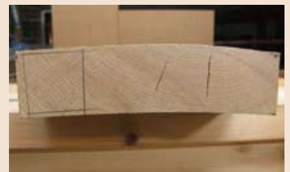
Cutting leg piece from the edge of the board gives diagonal annual rings
