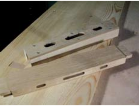
16 Back slat mortises and the jig used to create them
