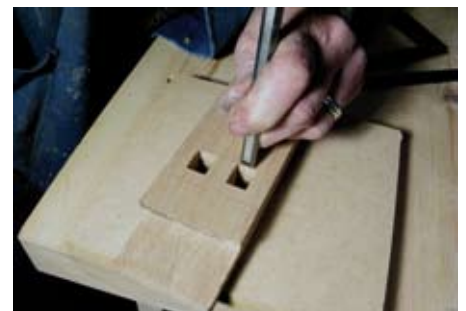
9 ... then a sharp chisel is used to open out the mortise
