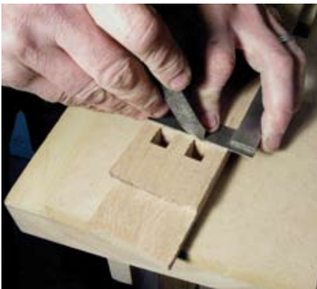
14 Use a sharp knife to mark for chiselling the outside of the through mortise
