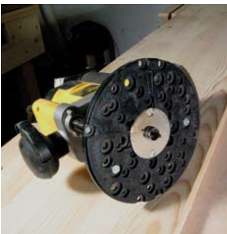
15 Trend Unibase with collar fitted to router
