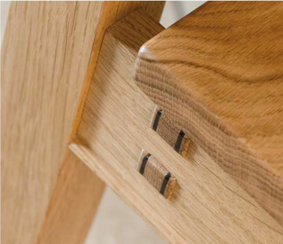
17 The tenons are formed on the back slats using a jig on the router table
