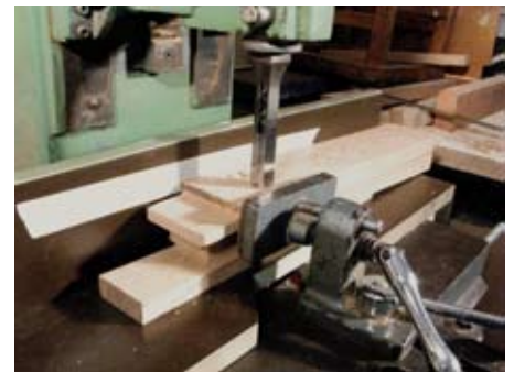
8 The through mortises are cut from both sides to avoid breakout...
