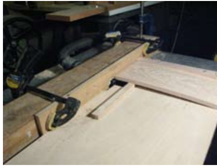
17 The tenons are formed on the back slats using a jig on the router table
