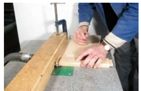
10 Cutting front rail tenons using simple board support
