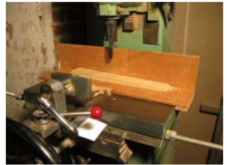
7 A shaped wedge as packing for the front leg mortising operation
