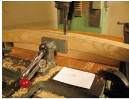
6 Cutting side rail mortises using the curved jig
