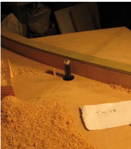
3 Shaping back leg on router table – the guide is removed for clarity
