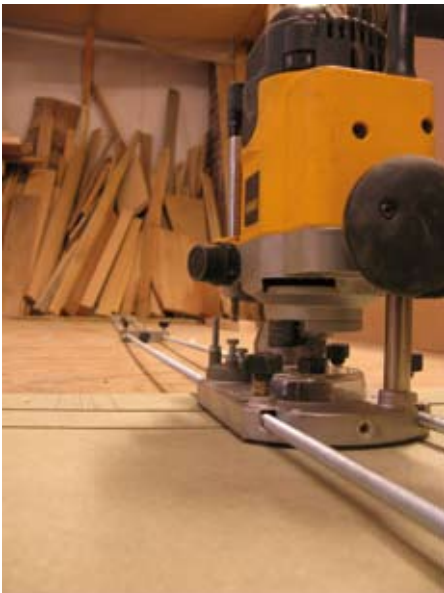
1 Setup used to cut curve for back leg template
