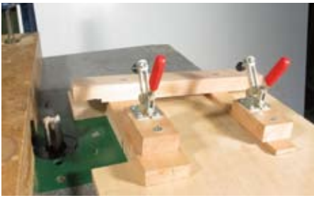
11 Jig used to hold side rails at correct angle for tenoning
