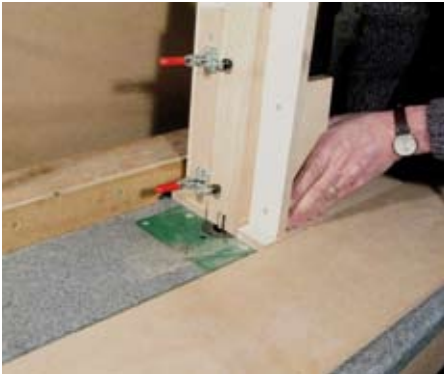
13 Jig used to cut tenons on back rail; note double fence to prevent wandering
