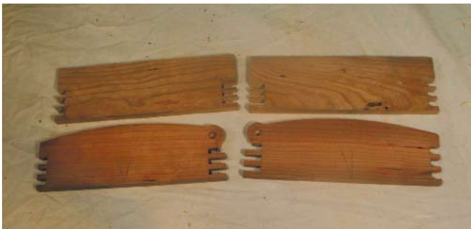
Box sides before shaping (top) and after shaping (bottom) – note over-length pins
