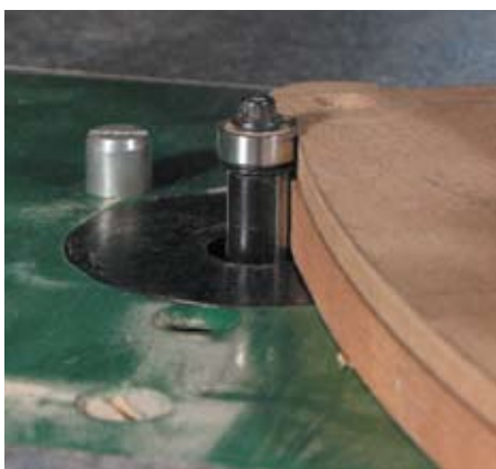
Shaping the panel side – end of cut. Note: the guard is removed for the photograph only
