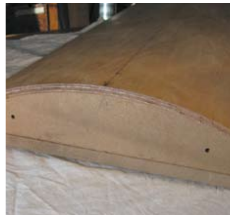
Former with outer layers fitted. Note centre line
