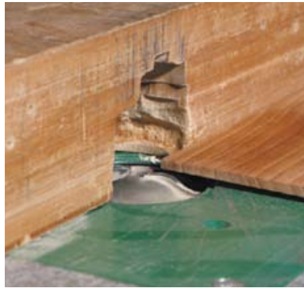
Fielding the bottom panel on the router table. Guard is removed for photograph only
