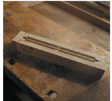
Box jig for holding the spine in order to rout the groove
