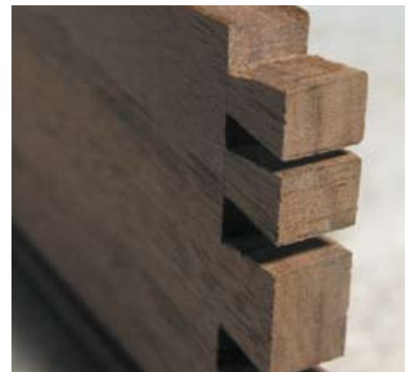
End of back piece showing the curved profile for the lid hinge
