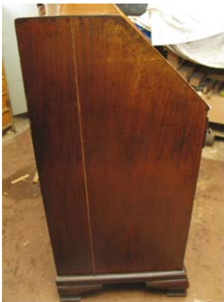
10 Vertical fillet fitted to left-hand side
