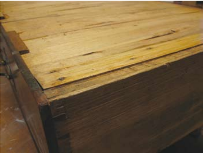
11 Worn and damaged drawer sides and nailed runner
