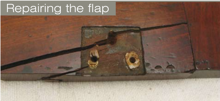
1 Damage to left hand of flap; note worn screw holes
