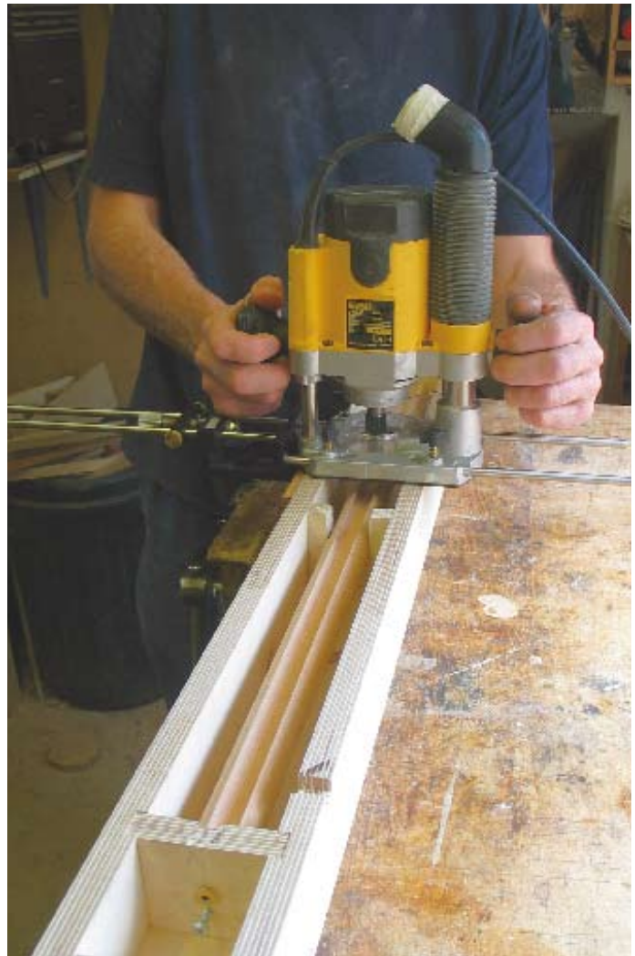
Routing the door column in the jig
