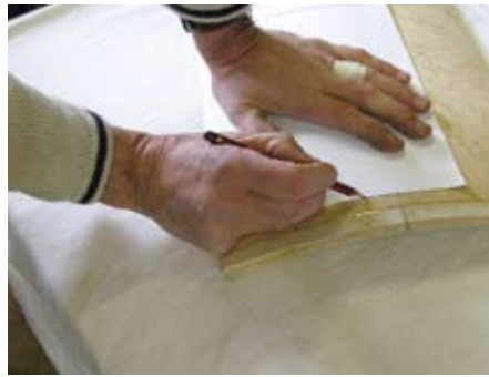
Using square paper to mark the end of the door panel
