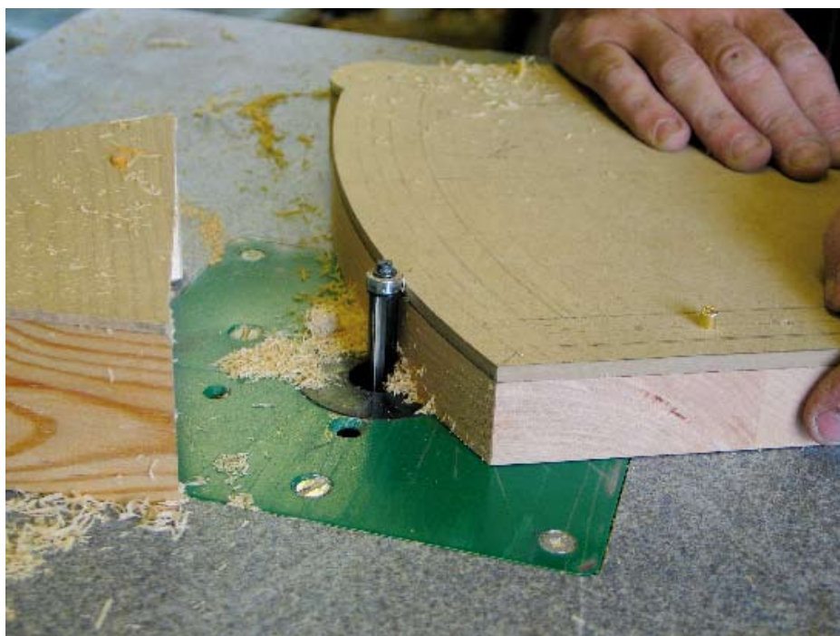
Shaping the cabinet bottom on the router table using a template secured with brass pins
