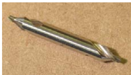
Engineering centre drill used to precisely locate the hole
