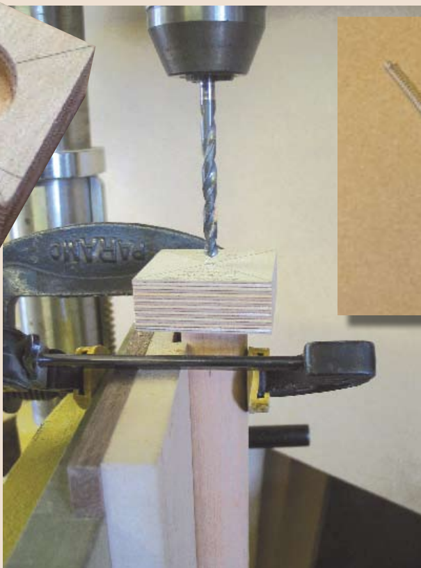
Far left: Detail of the column centre drilling jig
