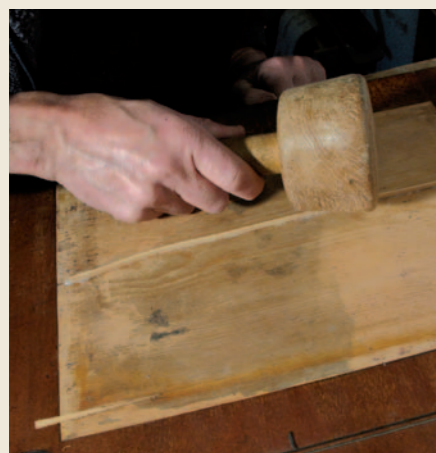
Cracks Tapping home a fillet into a crack in the substrate of the panel
